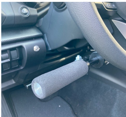
Figure 1: Hand Controls (Brake and Twist Throttle)
