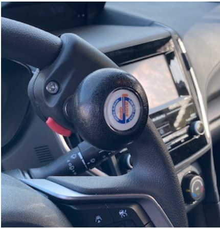
Figure 2: Steering Wheel Spinner Knob
